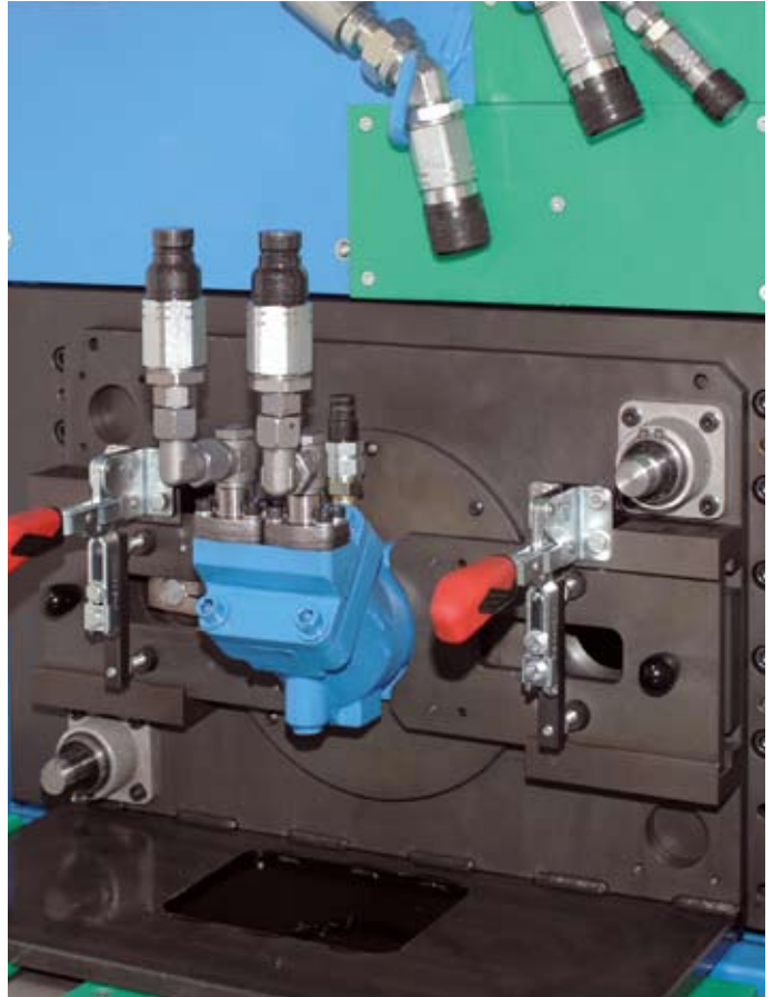
test bench for motors
